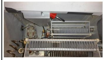
The RF deck with the changeover relay in the upper left corner. The red screw driver is over-riding the HV interlock during checkout.
