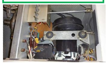
Here's the blower compartment. Blower and motor are on right (black stuff). The tube socket and boot are on discharge of blower and you can just see the tube on the other side of the aluminum partition. The ALC transformer is hiding in the lower right hand corner out of view.
