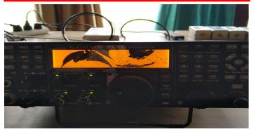
First 2427 QSOs uploaded to Club Log. Today, Yuris will finish low-band antenna and try to work lower bands later. One K3 transceiver was dropped while in transit and its display is damaged, so now frequency has to be set only from computer using CAT connection. Power outages happen quite frequently, and it takes time to start generators.
